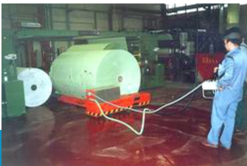
ROMEX® industrial floor coating for the use of air cushion transport systems in the paper and foil industry
