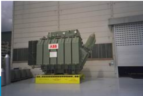
ROMEX® industrial floor coating for the use of air cushion transport systems in the transformer and generator industry
